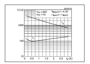
Figure 10. Resistive load switching time
